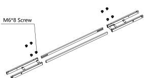
This step has been pre-installed before shipment, please check whether there is a lack of spare parts, and adjust the frame extension tube to the appropriate length.
